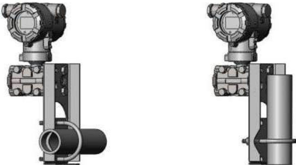
Pipe mounted flat bracket installation
